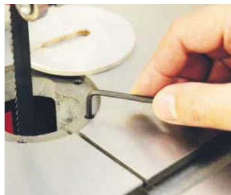
Height adjusting screws allow the insert to sit perfectly flush
